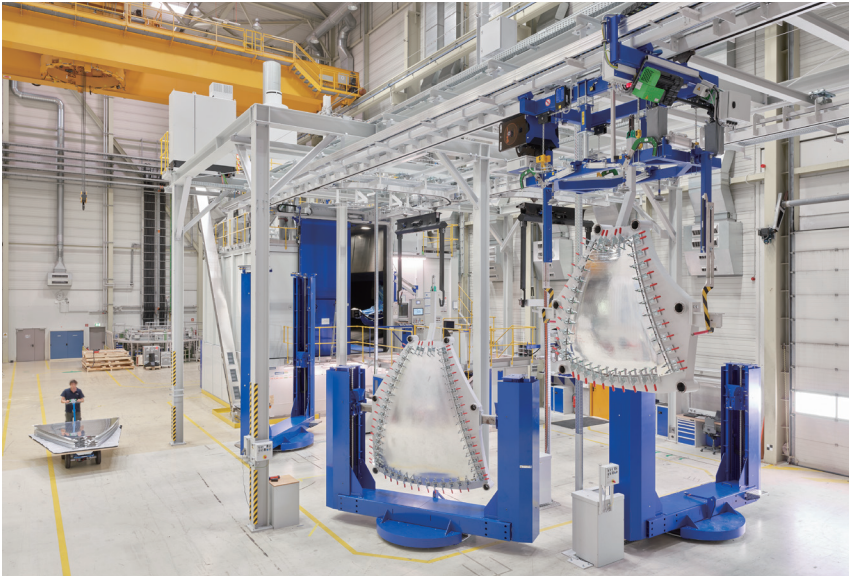
No touching of critical part zones thanks to automated transport and measurement processes
